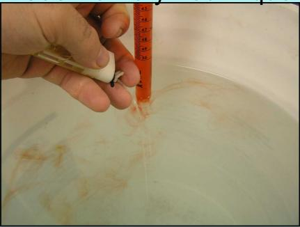
Notice the lighter never gets wet. In this case, red die is flowing out the bottom do to the fact water is being displaced
